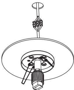
**B.** Before mounting the fitting, ensure that the surface being mounted to is flat and smooth to create a secure seal around the back plate.
