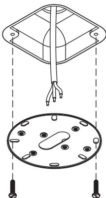
**B.** Make the electrical connection between the ceiling/wall and the fitting ensuring all wires are colour matched and the fitting is earthed correctly.
