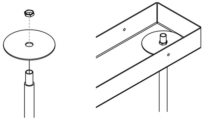
3. Attach the ceiling plate to the ceiling ensuring that you are using screws appropriate for the surface that you are mounting to, and with the electric cable centered with the hole in the middle of the plate.
