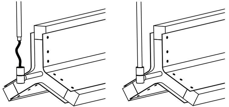
2. Remove the nuts and strengthening plates from the top of the drop rods and attach ceiling rose by placing over the drop rods and replacing the nuts and strengthening plates.
