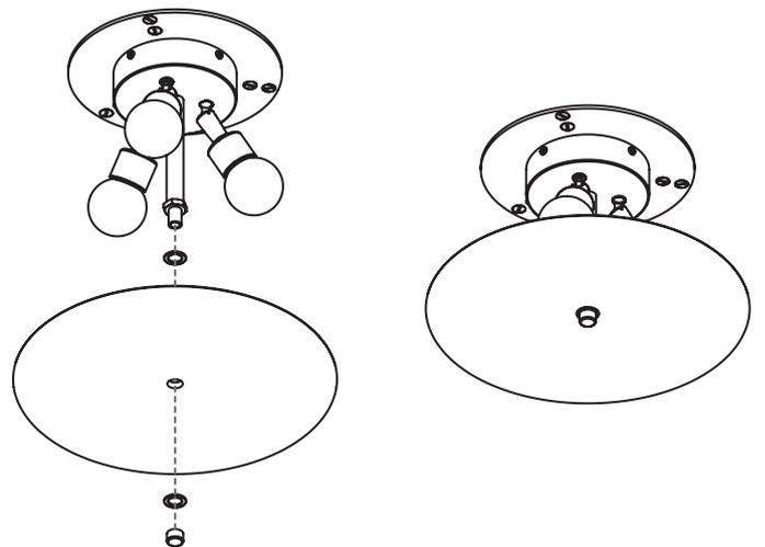
**7.** Mount the glass disks to the hooks located on the underside of the main body using the diagram.
