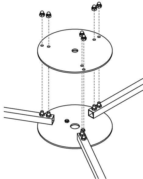
2. Remove the M10 nut from the bottom of the drop rod and place the brass disk onto the end, replacing the M10 nut.
