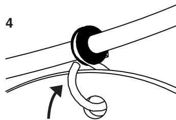
Using a pair of pliers, carefully open the glass mounting hooks ( **1** ) wide enough to fit the glass disks ( **2** ). Fit the glass disks to the hooks ( **3** ) carefully close the hooks with the pliers ( **4** ) taking care not to damage the glass or the fitting.
